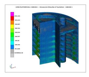
Strains, stresses and displacements are examined then in  $\mu$ ETA. Critical areas with high stress values can be identified and further analysis can be done for every case. Some results are presented below.
