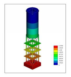
Setting the inertia relief parameter in NASTRAN to -2 there is no need of SPC use in the model and the platform remains unrestrained. NASTRAN will counteract any remaining resultant force or moment by applying inertial forces induced by an acceleration field. In this way, it is possible to have a static solution.
