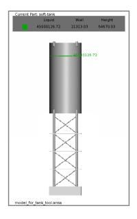
As a last step, buoyancy pressure is applied to every element below waterline, varying according to water depth. The results can be visualized through an element pressure graph. The resultant buoyancy force is calculated at about 41.86\*10<sup>7</sup> N.
