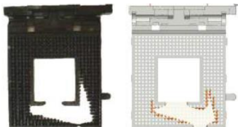
Moldex3D provides accurate simulations of filling patterns for plastic parts even with complicated geometry.
