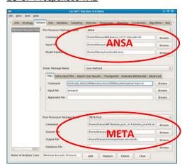
LS-OPT provides a direct coupling to ANSA and  $\mu$ ETA without the need for any scripting or customization. At the Solver Tab of LS-OPT, the user can define the pre- and post- processing sequence that will run in batch mode for each iteration. The design variables, defined in ANSA, are imported in LS-OPT and listed at the *Variables* tab. In the same
