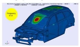
Responses can be defined using the run-time *Annotations*. This is a comprehensive tool for tracing results from the 3D models or 2D curves. Mathematical functions can also be applied to extract combined results.
