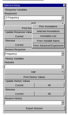
The OptimizerSetup User Toolbar has been developed in  $\mu$ ETA for the effortless extraction of responses and histories.
